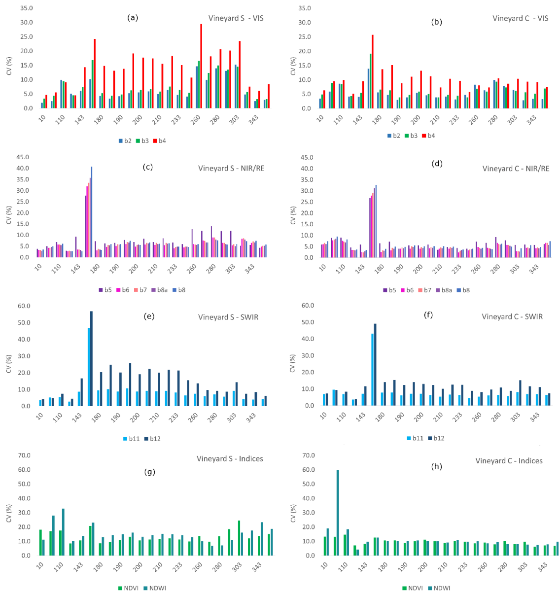
Figure 7. Coefficients of variation (CV) of covered vineyards (S and C) along the year (2016). CV concerns spatial distribution of band/index values within the vineyard. Values were computed at plot level for each date for all the considered S2 bands and for NDVI and NDWI indices. Figures (a,c,e) refer to vineyard S and show temporal trends of visible, NIR and SWIR bands, respectively. Similarly, figures (b,d,f) refer to vineyard C and show temporal trends of visible, NIR and SWIR bands, respectively. Figure (g,h) show temporal trends of spectral indices (NDVI, NDWI) for vineyard S and C respectively.
