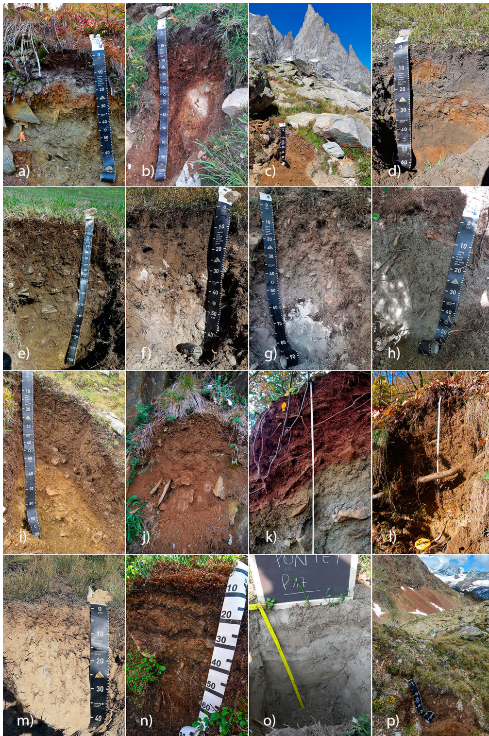
Figure 3. Examples of soil types belonging to the 16 CUs (Table 3). (a) CU1 – Albic Ortsteinic Podzol; (b) CU2 – Entic Ortsteinic Podzol; (c) CU3 – Umbric Entic Podzol; (d) CU4 – Protospodic Dystric Cambisol; (e) CU5 – Haplic Phaeozem; (f) CU6 – Calcic Kastanozem; (g) CU7 – Petric Calcisol; (h) CU8 – Calcic Regosol; (i) CU9 – Cambic Umbrisol; (j) CU10 – Eutric Skeletic Cambisol; (k) CU11 – Hypocalcic Cambisol (Rhodic); (l) CU12 – Dystric Cambisol; (m) CU13 – Eutric Regosol; (n) CU14 – Turbic Regosol; (o) CU15 – Haplic Fluvisol (Arenic); (p) CU16 – Dystric Leptosol.
