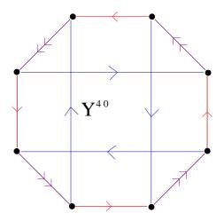
**Figure 8:** Quiver diagram for  $Y^{4,0}$ . Note that the superpotential terms are only quartic. Correspondingly, the nodes have precisely 2 incoming and 2 outgoing arrows. This quiver diagram is indeed a  $\mathbb{Z}_4$  orbifold of the conifold.
