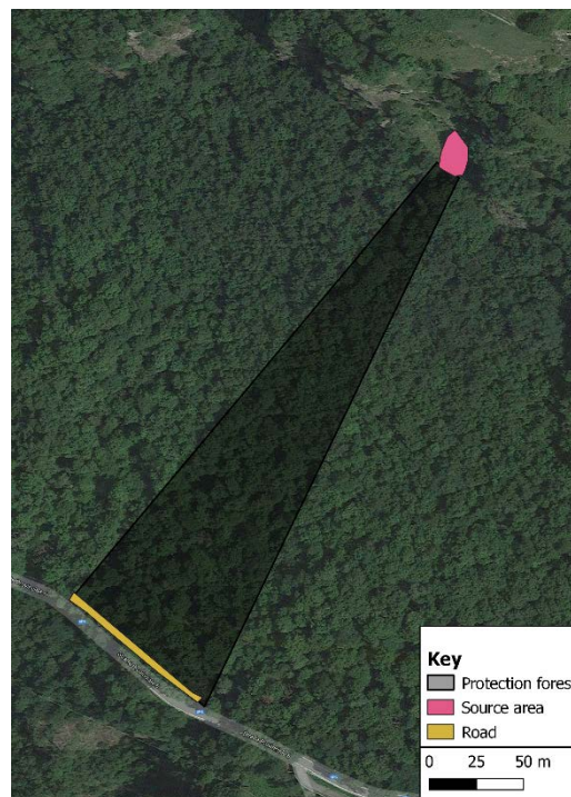
Figure 3 - Source area, protection forest and the asset to be protected (road).
