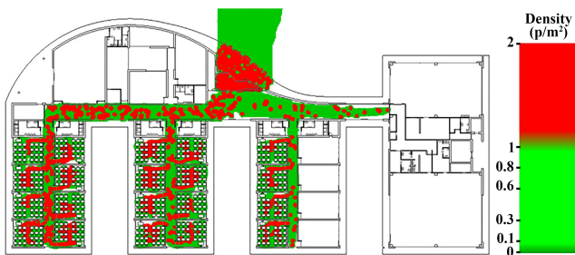
Figure 2: Density map resulting from crowd simulations on the primary school of Melzo.
