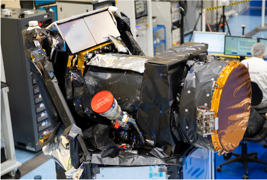
Fig. 7 Picture of the payload after integration on the platform with the star tracker optical heads (red covers). Image credits Airbus DS Spain.
