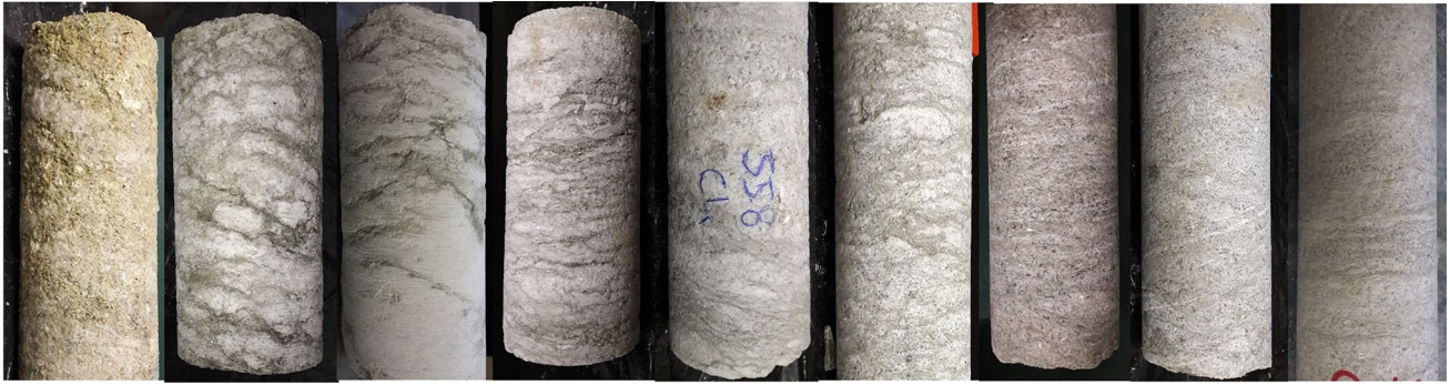
Fig. 2 Samples of branching selenite gypsum, underlining the mesoscopic heterogeneity of the material
