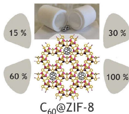
Figure 1. Mechanochemically synthesized C 60 @ZIF-8 crystalline materials containing 15, 30, 60, and 100 mol % of Buckminsterfullerene
