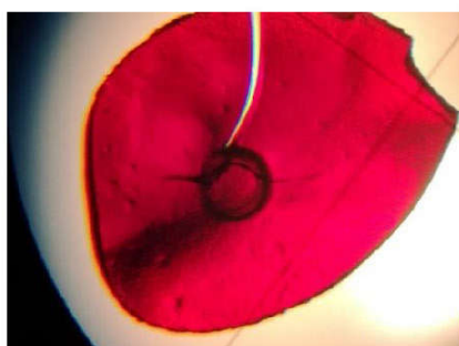
Fig. 1. Fe-BTC xerogel from the shrinking process during slow drying of gel at room temperature observed with an optical microscope.
