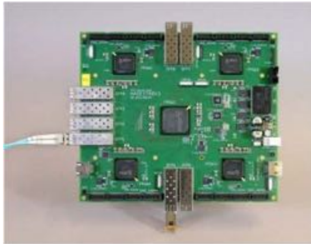
(a) The TRB3 is equipped with a central FPGA and four peripheral FPGAs near the corners.
