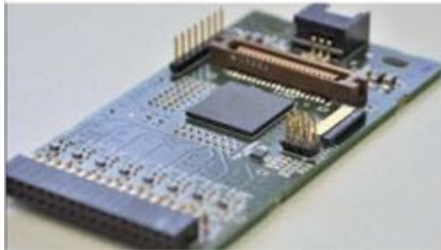
(b) The PADIWA front-end boards have connectors that plug in directly to the photon sensors.
