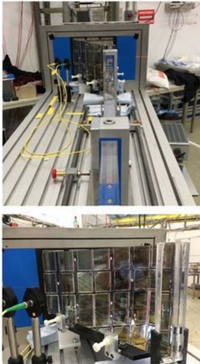
Figure 117. Photographs of the 2016 prototype in the T9 beam line: view along the length of the plate (top) and close-up of the coupling of the prism to the 2-layer cylindrical lens and to the 3 \times 3 MCP-PMT array (bottom).
