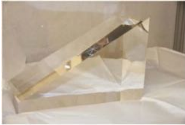
Figure 50. One of two solid fused silica expansion volume prototypes produced for the Barrel DIRC system tests with particle beams. This prism has an opening angle of 30^\circ , a width of 170 mm, and a depth of 300 mm.
