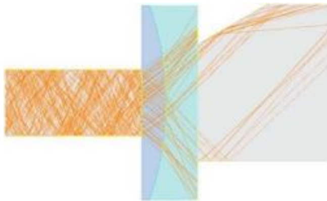
Figure 120. Close-up of the region of the 2-layer cylindrical lens in simulation for the 2016 configuration. The orange lines represent the Cherenkov photons originating from one \pi^+ with 7 GeV/ c momentum and 90^\circ polar angle.
