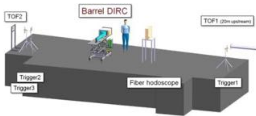
Figure 114. Detector setup during the prototype test in the T9 beam line at CERN in 2016 (not to scale).
