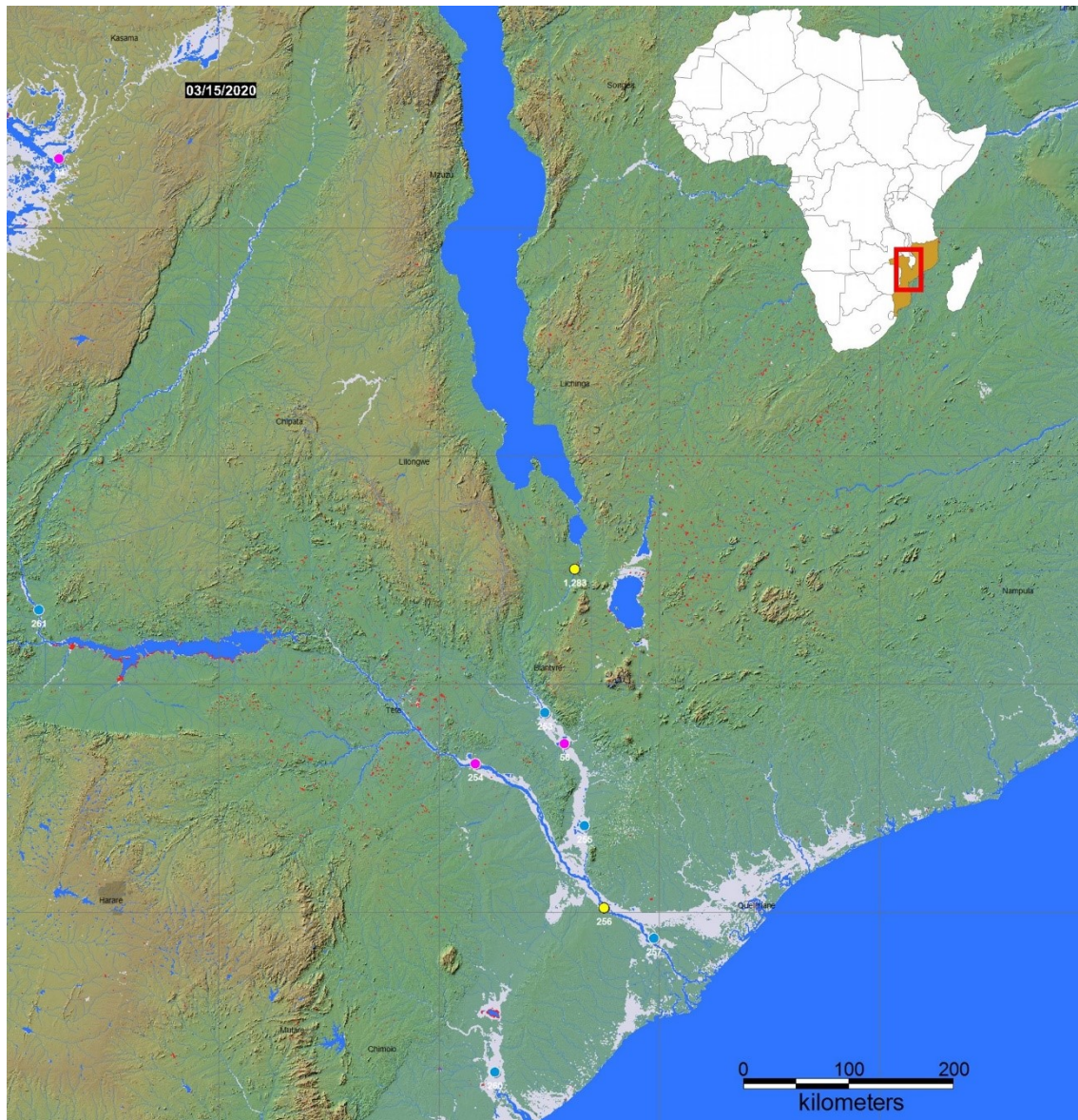
Figure 6. Mozambique: large scale flood mapping from various satellites, including MODIS, Landsat and ESA Sentinel-1. Blue areas: mean annual flood. Red areas: flooding in excess of mean annual flood. Light gray areas: maximum observed flooding, 1993 - Present. The colored dots are interactive and contain River and Reservoir Watch information.
