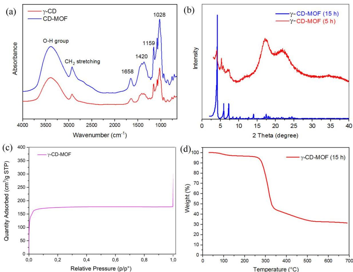
**Figure 2:** (a) FTIR spectrum, (b) PXRD patterns, (c) N<sub>2</sub> adsorption/desorption isotherms and (d) TGA curve of synthesized CD-MOF.
