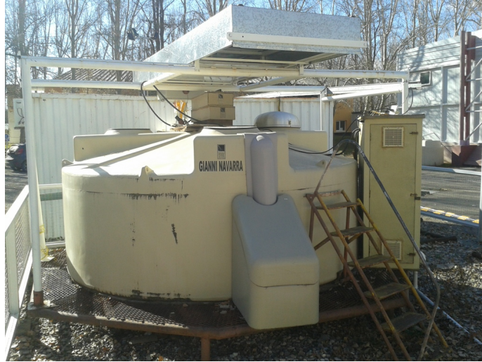
Figure 1. A photograph of the experimental setup in Malargüe, showing the aluminum box with the top RPC installed above the Gianni Navarra WCD. The bottom RPC is under the mesh support structure of the WCD and is not directly visible.
