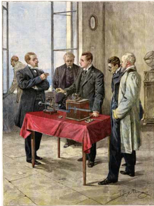
Fig. 14 Marconi during the English Channel experiment. This illustration, published on the Italian weekly magazine La Domenica del Corriere on April 23, 1899, mimics the famous Strand magazine photograph, with Righi's oscillator on the left and Marconi's closed box on the right [31]
