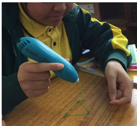
Fig. 1 Using a 3D Printing Pen to construct models in 3D
