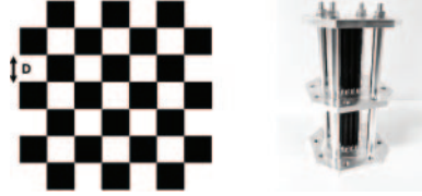
Fig. 1. – Left: cross section of the ANET collimator geometry. In white the “air” channels, in black the absorbent material channels. Right: a picture of the ANET collimator prototype assembled at the Frascati National Laboratories (LNF).
