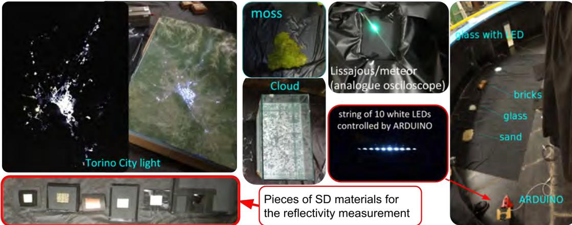
Figure 4: Light sources and materials to reproduce phenomena that Mini-EUSO can observe are visible. Reflections of materials that are often present in space debris (SD) have also been tested.
