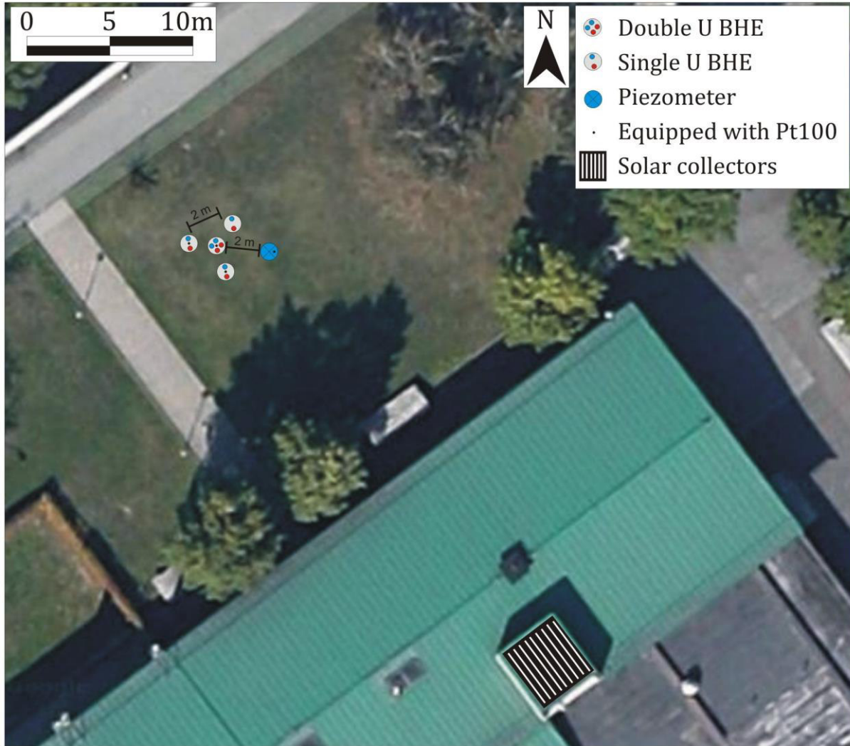
Fig. 9 - Satellite image [51] of the test site area. The arrangement of the BHEs and the monitoring hole are reported with the indication of the boreholes equipped with temperature sensors. The green roof is that of the Topography building where the solar collectors are placed.
