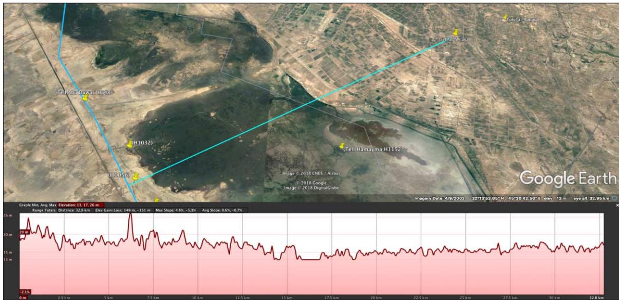
Fig. 3. Elevation profile of reconstructed Tabbi-Mama canal ©Google.
