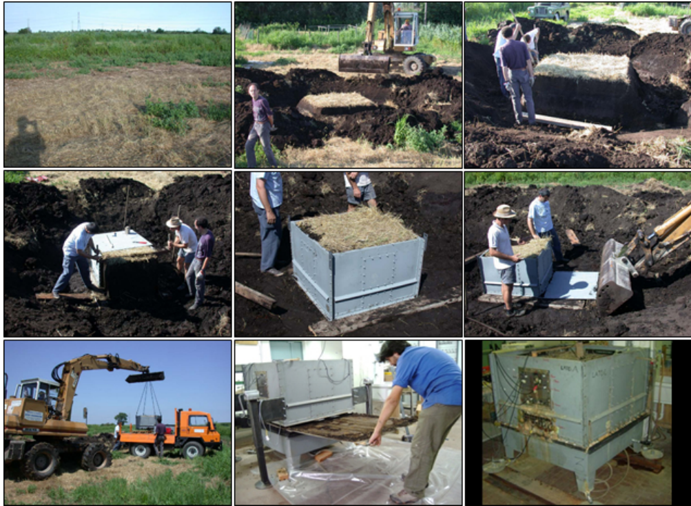
Figure 2. Successive phases of the monolith collection, from the undisturbed sampling zone to the sample removal with a steel box structure built around the soil monolith, until the final lysimeter arrangement in laboratory.
