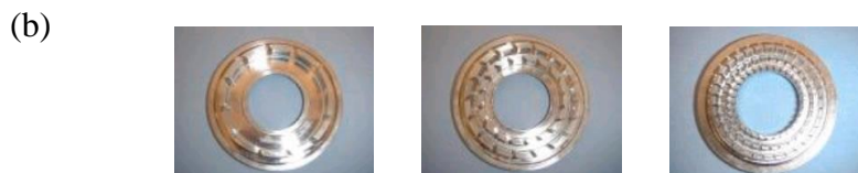
349 Figure 1. (a) HSM (Magic-Lab, IKA) and (b) Three types of rotor; coarse, medium and fine 350 rotor, respectively.
