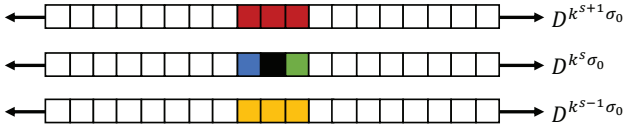
Fig. 8: A sample candidate feature point, \mathcal{F} , (solid black) and its neighbors in adjacent scales “ s + 1 ” (red) and “ s - 1 ” (yellow) and in time “ t - 1 ” (blue) and “ t + 1 ” (green)
