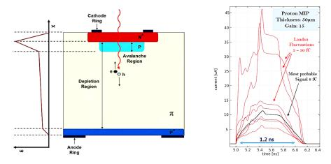
Figure 1: LGAD structure and signal shape.
