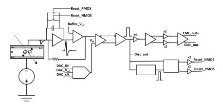
Figure 2: CSA-based architecture
