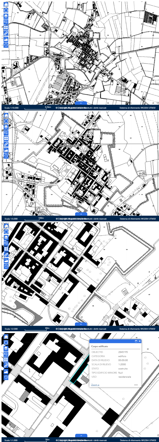
Figure 7. A portion of the DBTR in the historical town of Sabbioneta (province of Mantua) is displayed at four different scales in the Geographic Viewer. Objects' properties can be displayed at visualization scale 1:1,000.
