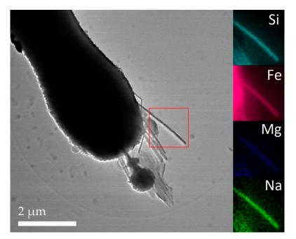
**Figure 6.** STEM image of crocidolite fibres. The red square identifies the area selected to carry out the EDX mapping. The fibre inside the red square is the same as in Figure 5. The STEM-EDX maps on the right side show the spatial distribution of Si (turquoise), Fe (red), Mg (violet), and Na (green). The maps were generated after background subtraction performed on the spectra obtained in the studied region of interest (ROI).
