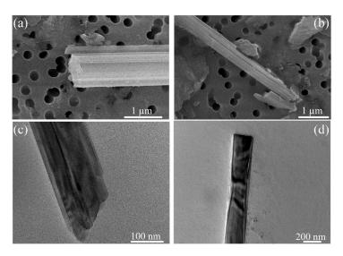
**Figure 3.** (a) High-resolution FEG-SEM image of an amosite fibre; (b) high-resolution FEG-SEM image of bundles of crocidolite fibres; (c) TEM image of a crocidolite fibre with stepped edges; (d) TEM image of an individual crocidolite fibre showing characteristic diffraction contours.
