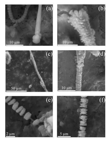
**Figure 9.** FEG-SEM images of asbestos bodies found in the lung of the human subject. (**a**) Typical sub-rounded AB segments at the tips of fibres. (**b**) The AB at the fibre tip showing typical multiple sequences of coatings. (**c**,**d**) ABs showing a habit in which the individual segments are fused (or partially-fused) together; (**e**) disc-shaped beaded segments; (**f**) disc-shaped segments partially-fused.
