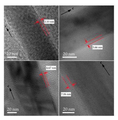
**Figure 7.** Selected examples (HRTEM images) of four highly crystalline, non-coated crocidolite fibres with a very thin amorphous layer on their surface. Red arrows and red lines highlight the amorphous layer. c = c-axis of crocidolite. The crocidolite fibre shown in the right top box is the same as shown in Figure 5. The images were acquired after a check of the stability of fibre under an electron beam. The black arrow indicates the direction of the crystallographic c-axis.
