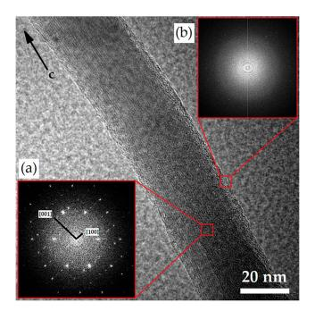
**Figure 5.** High resolution TEM image of a highly crystalline crocidolite fibre after a residence of ~40 y in the lung of the subject. (a) FFT pattern of the core of the fibre; (b) FFT pattern of the thin amorphous surface layer. The black arrow indicates the direction of the crystallographic c-axis.
