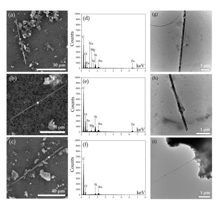
**Figure 2.** (a) FEG-SEM image of a crocidolite fibre; (b) FEG-SEM image of an amosite fibre; (c) FEG-SEM image of a silica-rich relict of chrysotile; (d) SEM-EDX spectrum of the fibre shown in (a); (e) SEM-EDX spectrum of the fibre shown in (b); (f) SEM-EDX spectrum of the fibre shown in (c); (g) STEM image of an individual crocidolite fibre with columnar habit; (h) STEM images of a prismatic individual crocidolite fibre; (i) STEM image of a thin crocidolite fibre.
