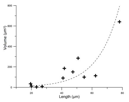
**Figure 10.** Scatter plot showing the volume of the ABs vs. the length of coated fibres. Dashed line represents an exponential fitting function ( $R^2 = 0.70$ ) to the data points.
