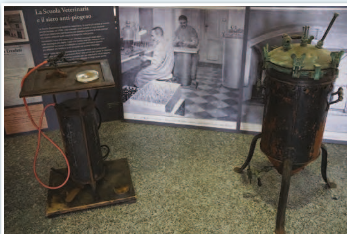
Figure 3. An old autoclave and a blowpipe for the production of anti-pyogenic serum during the WWI.
