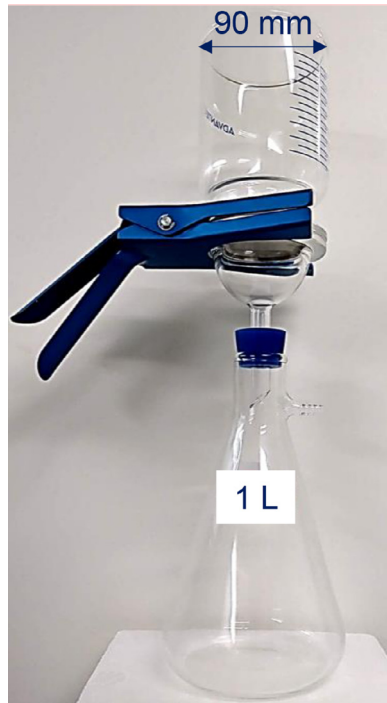
Fig. 1. Vacuum-filtration flask used for particle preparation. This system included a 1 L glass Büchner flask (bottom), a 90 mm diameter stainless-steel filter support housed in a glass base, and a 1 L glass Büchner funnel (top).
