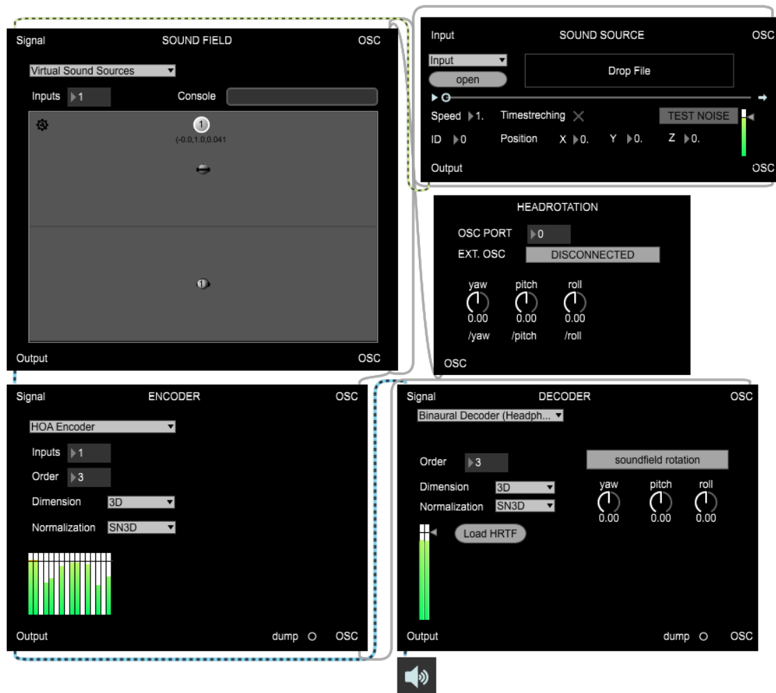
Figure 2. Spatial audio pipeline using IVES. The example shows a simple simulated sound field with one virtual sound source. It is based on 3rd order HOA rendering with binaural reproduction. It consists of a virtual sound field module with a single sound source module as audio input and the head rotation module for 3DoF motion tracking. The audio stream and position data from the sound field module is then spatialized using the en- and decoder modules.
