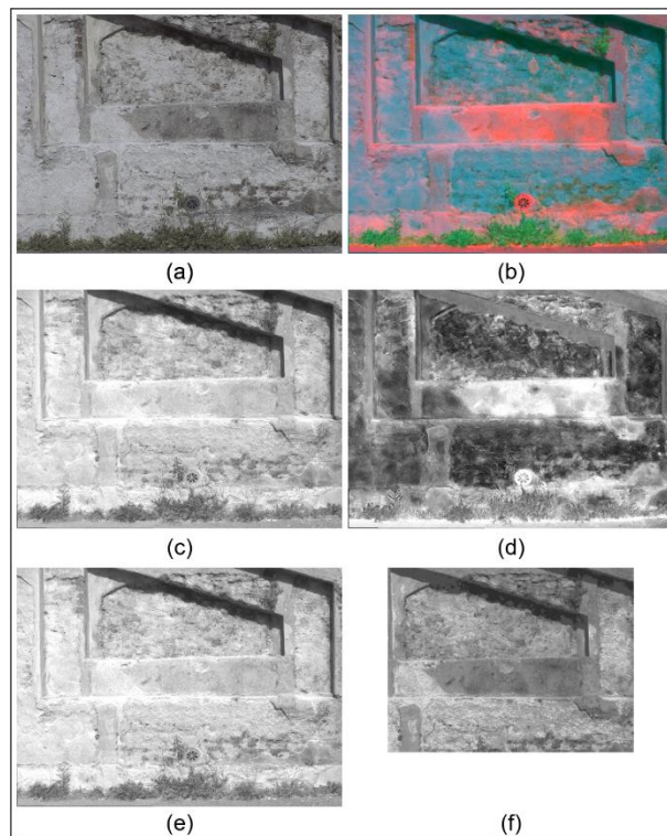
Figure 5.45. Castello del Valentino riverside façade multiband results: (a) cropped VIS image; (b) TIR-NIR-red false-color composite; (c,d) principal component analysis—first and second component; (e) Fourier transform; (f) quantized image.
