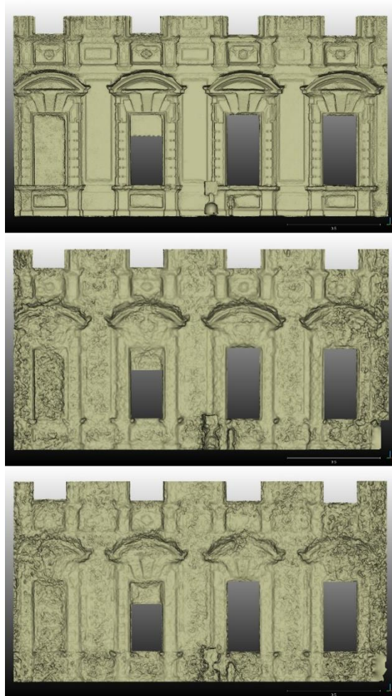
Figure 5.7. Façade models produced by Canon Rebel-SL1 and FLIR T1030sc optical imagery (top), FLIR T1030sc optical imagery (middle), and FLIR T1030sc thermal-infrared imagery (bottom).
