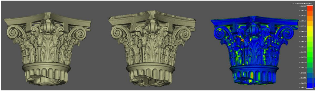
Figure 5.17. Scanning results. Untextured Stonex F6 SR mesh (left), untextured FARO Focus 3D X 330 mesh (center), and scalar field mapping of Hausdorff distances; maximum visualized distance 1 cm.
