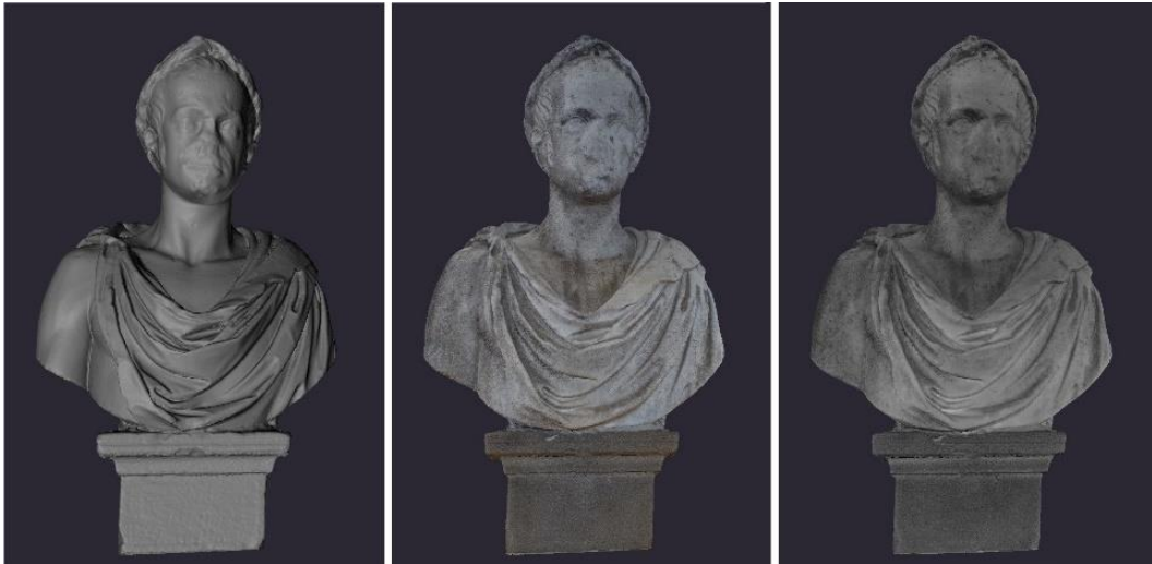
Figure 4.38. Digital models produced with image-based techniques: untextured (left), textured with RGB imagery (center), and with NIR imagery (right).
