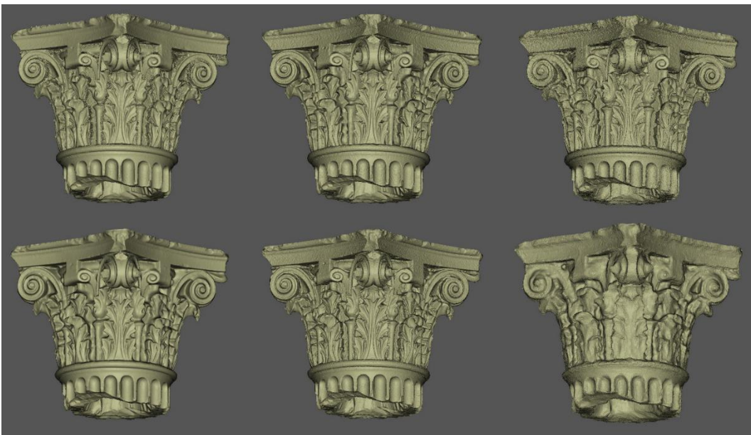
Figure 5.23. Untextured photogrammetric meshes of the capital replica from dataset 5, (from left to right, and from top to bottom): AMP, FZA, P4D, RCP, VCM, R3D.
