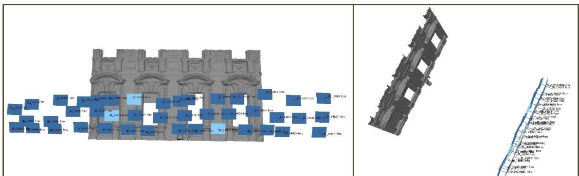
Figure 5.4. Visualization of the thermal image acquisition geometry.
