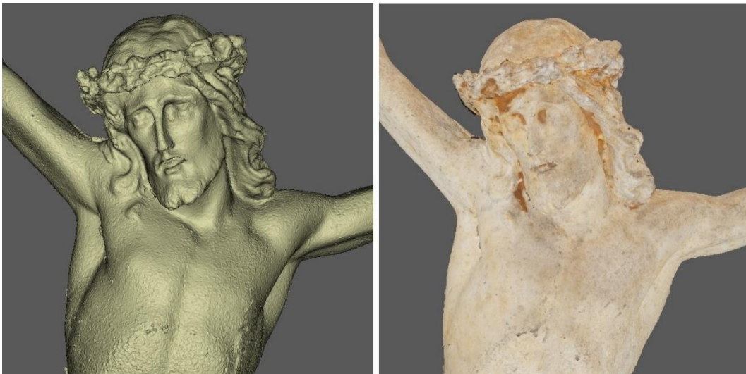
Figure 5.28. VCM-produced mesh from dataset 9 (smartphone camera).
