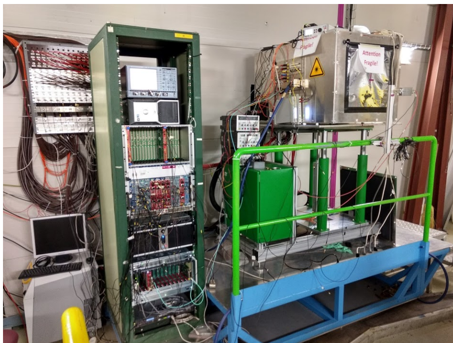
Figure 3.13: Picture of the test beam setup: the digitizer is on the left, while on the right there is the box in which the crystal matrix, the VFE and FE boards are installed.
