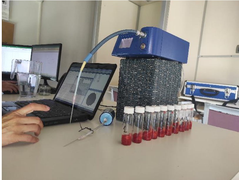
Figure 4.3: PEN e-nose during an analysis of a group of strawberries (10 vials).
