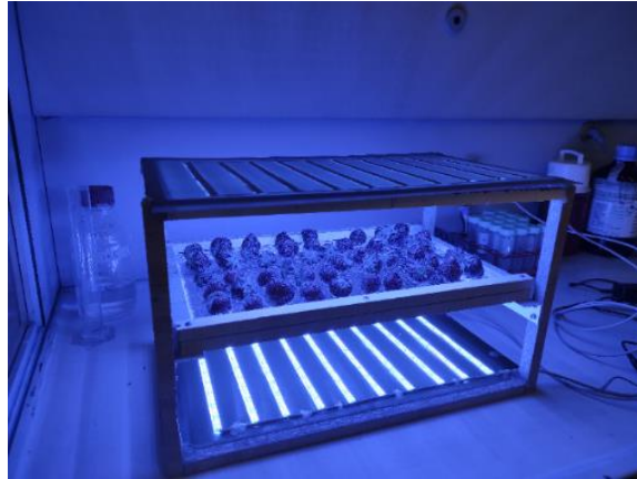
Figure 2.4: Irradiation chambers using LED (LES Flex Strips LEDYDEL IP64, Turin, Italy).
