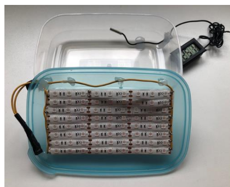
Figure 3.1: Container containing the LEDs for photodynamic treatment.
