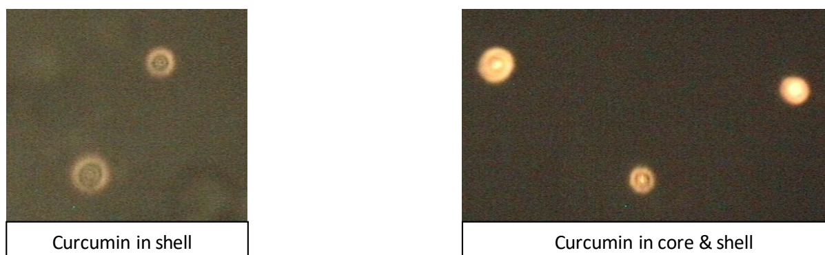
Figure 5.4: Morphological representation by fluorescence microscopy shows curcumin conjugated chitosan shelled NBs with (right) and without (left) curcumin in the core.
