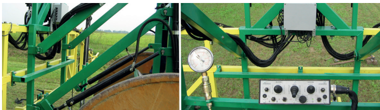
Fig. 7 – Pipes and hoses for hydraulic transmission (Photo: MAR snc)
