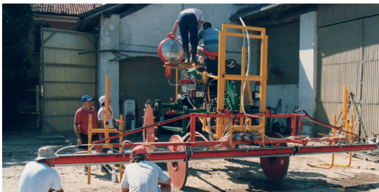
Fig. 10 – Example of vertical position control (Photo: G. Carezzo)
