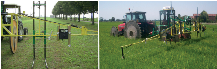
Fig. 4 - Example of weed wiper (distribution of herbicide not diluted using a cord – Type “B” – Photo: MAR snc).
