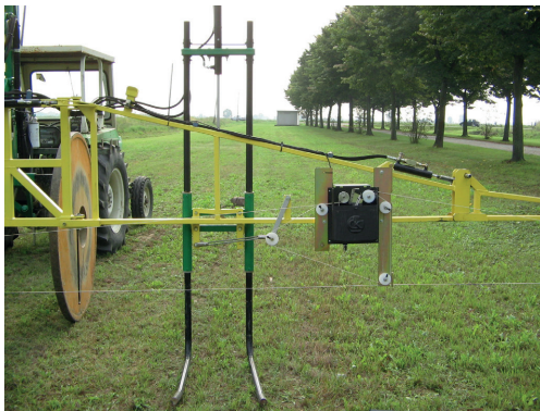
Fig. 11 – Example of device for damping unintended boom movements, slope compensation and stabilization system (Photo: MAR SNC)
