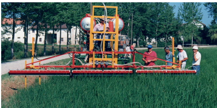
Fig. 2 – Example of weed wiper (distribution of mixture concentrated – Type “A”). (Photo: G. Careno).
