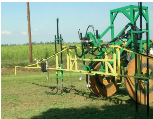
Fig. 9 – Example of stable boom (Photo: MAR snc)
