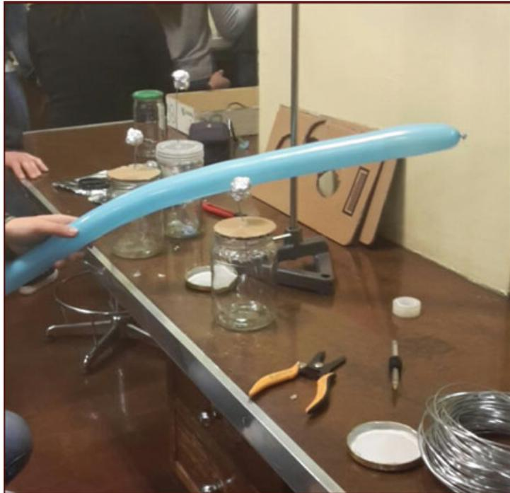
Through the construction of a rudimentary electroscope, inspired to those displayed in the collection, the students experience the struggle for arriving at a quantification of electricity and to the concept of electric charge (see Fig. 5).
