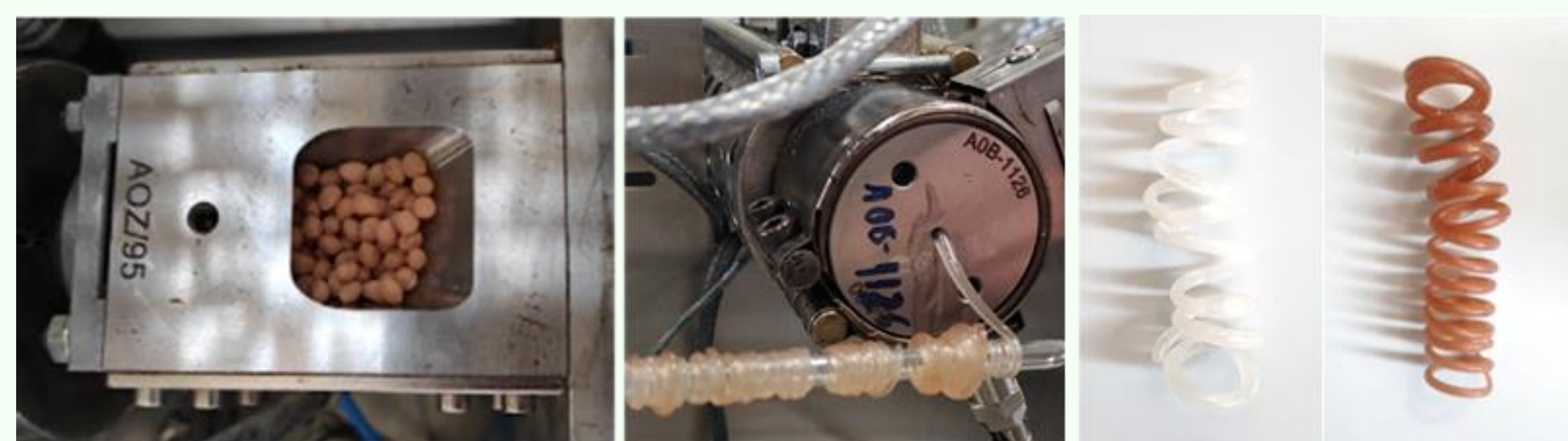
Main steps of blend preparation: (a) PEAA beads coated with \beta -CD/CPPE before extrusion (b) extrusion of the \beta -CD/CPPE-PEAA blend, and (c) the obtained blended PEAA: \beta -CD-PEAA (left) and \beta -CD/CPPE-PEAA (right) for comparison
