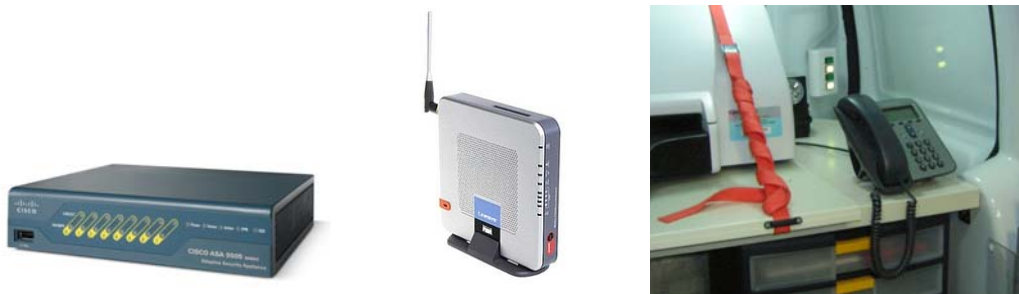
Fig. 5 - Firewall Cisco Systems – asa5505 – Router Cisco Systems – Wrt54g3g – telefono.
