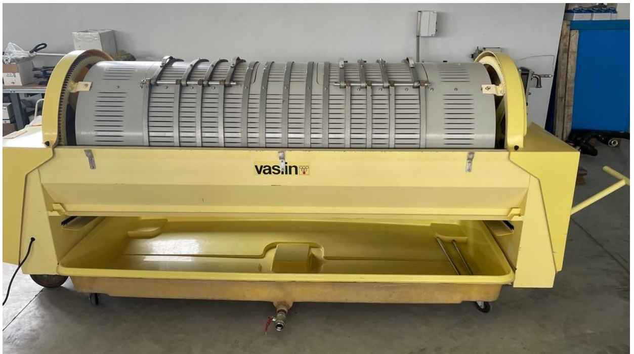
Figure 14. Vaslin Veritas 15 (Vaslin S.r.l.) grape pomace press.
