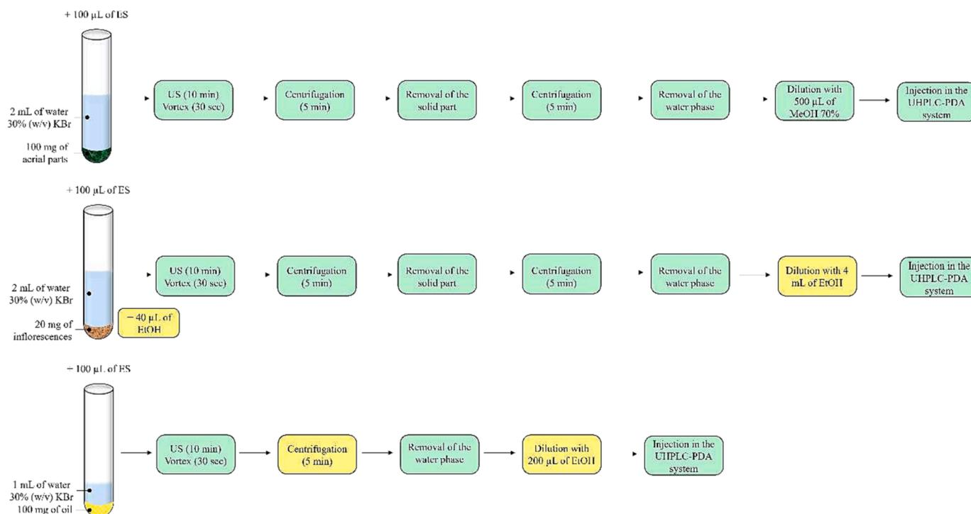
**Fig. 2.** Ultrasound-assisted dispersive solid-liquid microextraction method optimized for the analysis of different hemp products (aerial parts, inflorescences, and CBD oil). The differences between the procedures are highlighted in yellow. (For interpretation of the references to color in this figure legend, the reader is referred to the web version of this article.)
