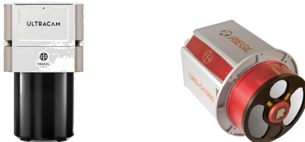
Fig. 1. Main devices used for the photogrammetric and LiDAR acquisitions: Vexcel UltraCam Eagle Mark 3 and Riegl LMS-Q1560
