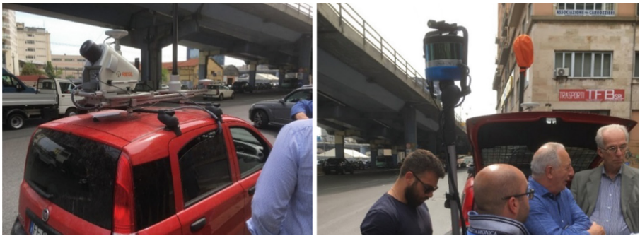
Fig. 3. Main devices used for MMS (Mobile Mapping System) acquisitions: Videocar equipped with the Vux1 LiDAR sensor and the Ladybug camera (on the left) and the Gexcel Backpack with the Velodyne LiDAR sensor (on the right)
