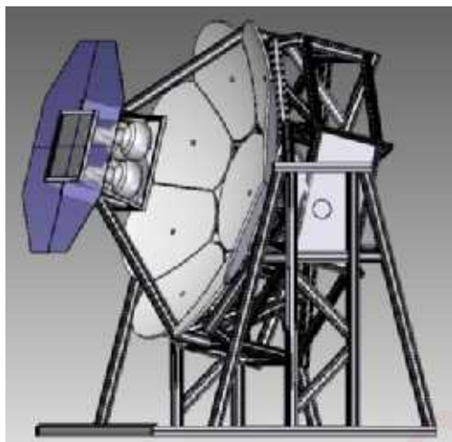
Figure 76: Concept of a fluorescence telescope frame, showing four PMTs at the focus of a 1.6 m diameter segmented mirror. The support structure is made from aluminium profiles. The UV band-pass filter can be seen attached to the periphery of the camera box.
