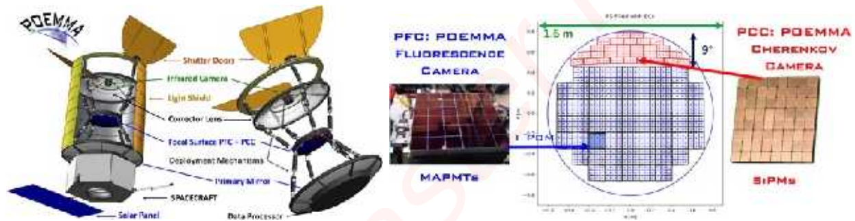
Figure 67: Left: Schematics of a POEMMA satellite and the Schmidt telescope consisting of a 4-m diameter primary mirror, 3.3-m diameter corrector plate, and 1.6-m diameter focal surface comprised of 126,720 pixels in the POEMMA Fluorescence Camera (PFC) and 15,360 pixels in the POEMMA Cherenkov Camera (PCC). Several components are detailed in the schematic including infrared cameras which will measure cloud cover within the 45^\circ full FoV of each telescope during science observations. Right: The layout of the hybrid focal plane of a POEMMA Schmidt telescope. The majority of the area is comprised of PFC MAPMT modules with a UV filter to record the 300–500 nm air fluorescence light in 1 \mu\text{s} snapshots. The PCC is comprised of SiPM pixels whose 300–1000 nm wavelength response is well-matched to that from the EAS optical Cherenkov signals and are recorded with 10 ns cadence. From Ref. [25]
