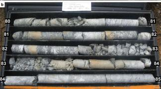
Fig. 6 - Core samples resulting from drilling in the Branega Fault Zone. a) Core samples of drill hole B1 taken at depth between 60 and 65 metres in the Branega Valley: at about 62.30 m depth, foliated cataclastic calc-schists make a transition to the underlying brecciated serpentinites (Acquasanta breccia); b) Core samples of drill hole SGG6 taken at depth between 80 and 85 metres: a calc-schist tectonic breccia and a gouge underlie brecciated serpentinites.
