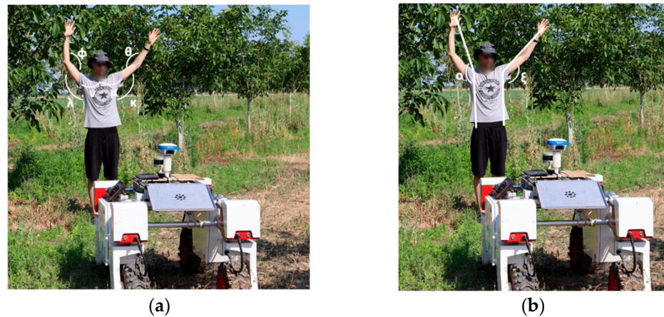
Figure 4. Depiction of the examined anthropometric parameters, namely the relative angles of both hands in relation to (a) the shoulders ( \hat{\kappa}_{left\ shoulder} and \hat{\lambda}_{right\ shoulder} ), the elbows ( \hat{\theta}_{left\ elbow} and \hat{\phi}_{right\ elbow} ), the chest ( \hat{\mu}_{left\ chest} and \hat{\nu}_{right\ chest} ) and (b) the torso ( \hat{\xi}_{left\ torso} and \hat{\delta}_{right\ torso} ).
