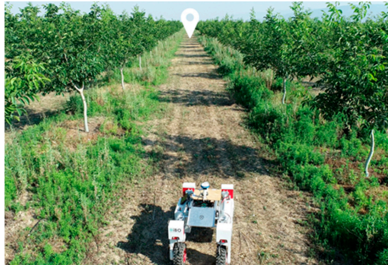
Figure 8. Image from the UGV autonomously navigating within the orchard toward a predefined site indicated by the map location sign marker.
