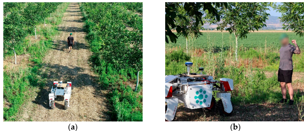
Figure 7. Images from the experimental demonstration of the “following” scenario in an orchard showing (a) the UGV following the locked participant while maintaining a safe speed and distance and (b) the participant asking the UGV to pause the following mode.
