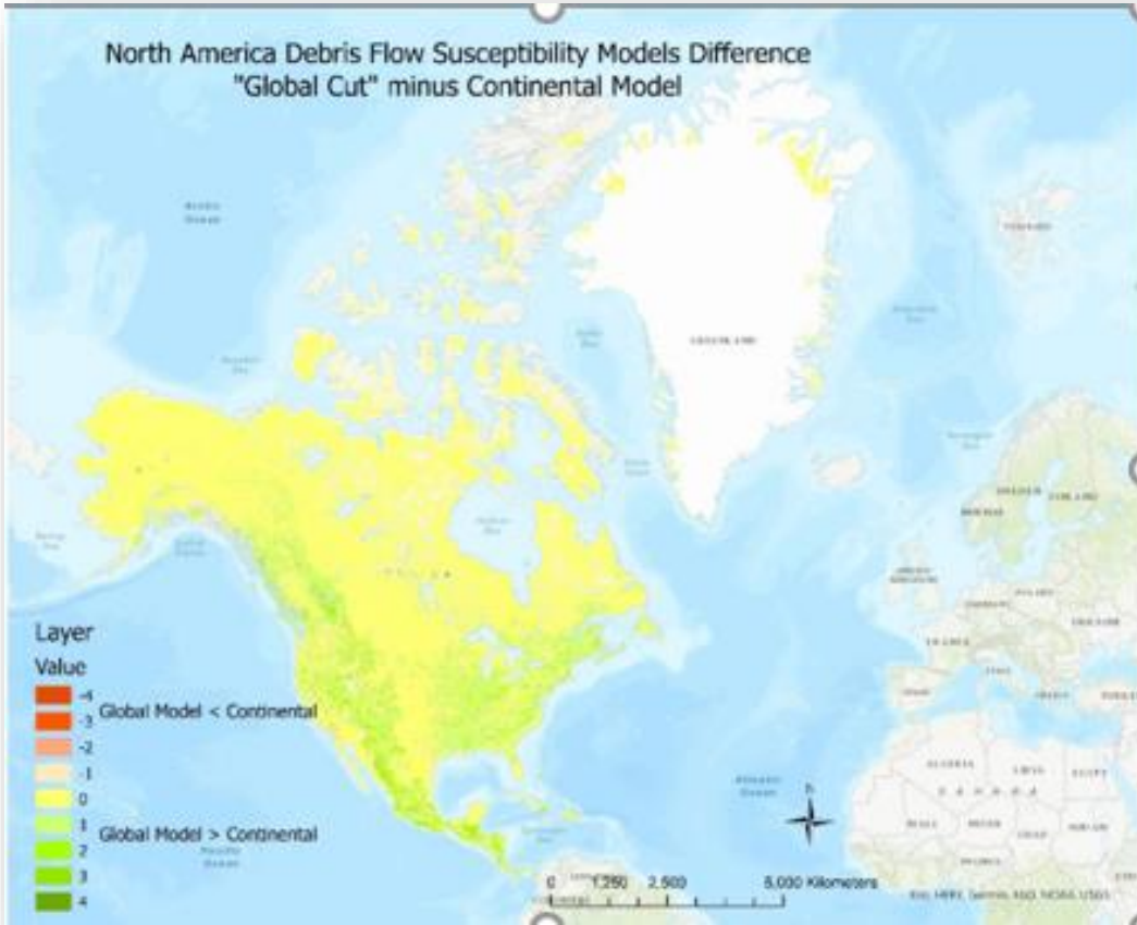
Figure 7.12 North America debris flow susceptibility difference map. Global cut model minus continental model. Positive numbers represent areas where the global model susceptibility is higher than the continental model, negative numbers represent areas where the continental susceptibility is higher.
