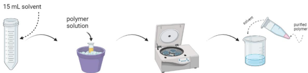
Figure 3. Illustration of purification steps. Purification occurs via precipitation. The polymer solution is dropwise pipetted into the solvent, which is already placed in an ice bath. After centrifugation and removal of the supernatant, the polymer is now purified.
