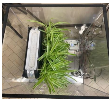
Figure 1: Top view of the chamber with the biofilter module, the heater and the NETPID sensor.
