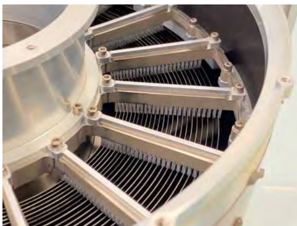
Figure 2.4: IXPE Mirror Module Assembly rear view showing the 24 nichel/cobalt nested mirrors.
