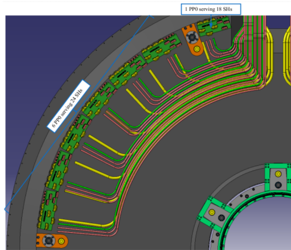
Figure B.2: High- and low-voltage lines in the outer edge of an ETL quarter-disk. PP0 modules (green) are well visible.
