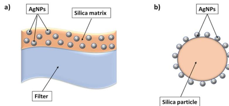
**Figure 4.** Comparison between two different silver–silica systems: (a) nanostructured silica composite coating containing silver nanoparticles; (b) silica particles decorated with silver nanoparticles.
