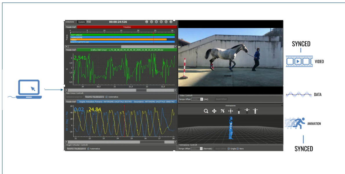
Fig 14. Motion analysis software. Top left of the picture showing raw data from a sensor; bottom left angle/time diagram of sagittal plane motion of metacarpo phalangeal joint of a right front limb (blue) and left front limb (yellow) simultaneously
