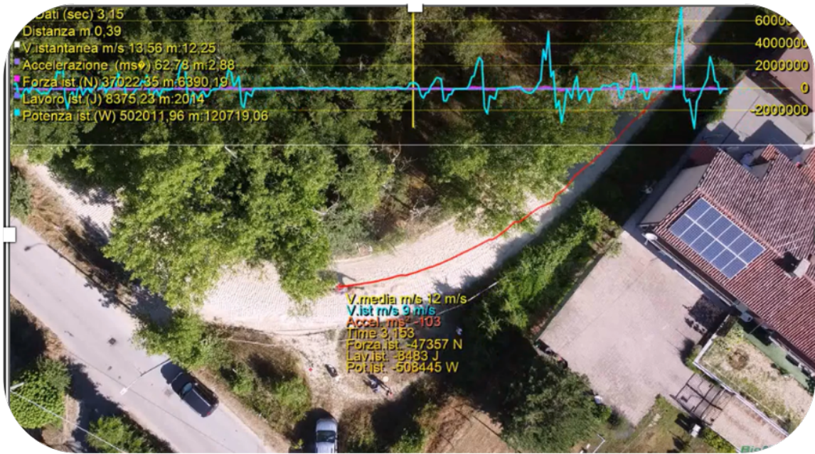
Fig 33. Calculation of instant velocity and acceleration from the drone on curve
