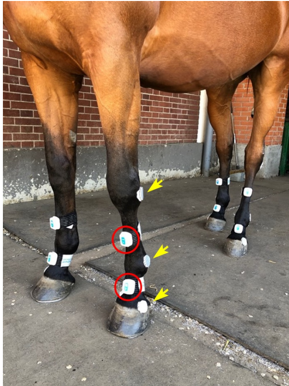
Fig 18. Placement of IMUs (red circle, identified only in one limb) and optical markers (yellow arrows, OMC technology) on equine distal limbs for data acquisition. The IMUs were fixed to the dorsal metacarpus/metatarsus and to the dorsal aspect of the pastern in the four limbs by means of plastic docking bases attached to elastic bands. Optical markers were glued to the skin on the lateral aspect of the joints studied.
