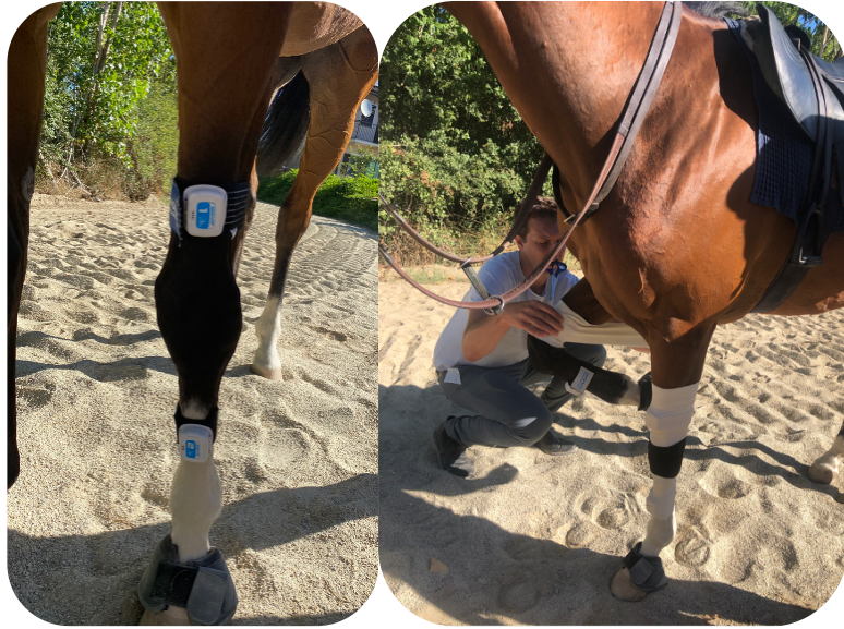
Fig 31. Positioning of the IMUs over the carpal joint
