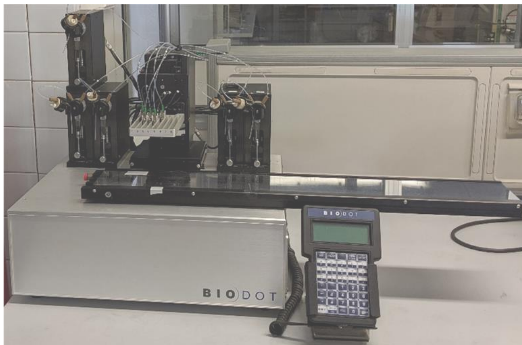
Figure 1.3. BioDot XYZ3050 platform equipped with five BioJet Quanti™.
