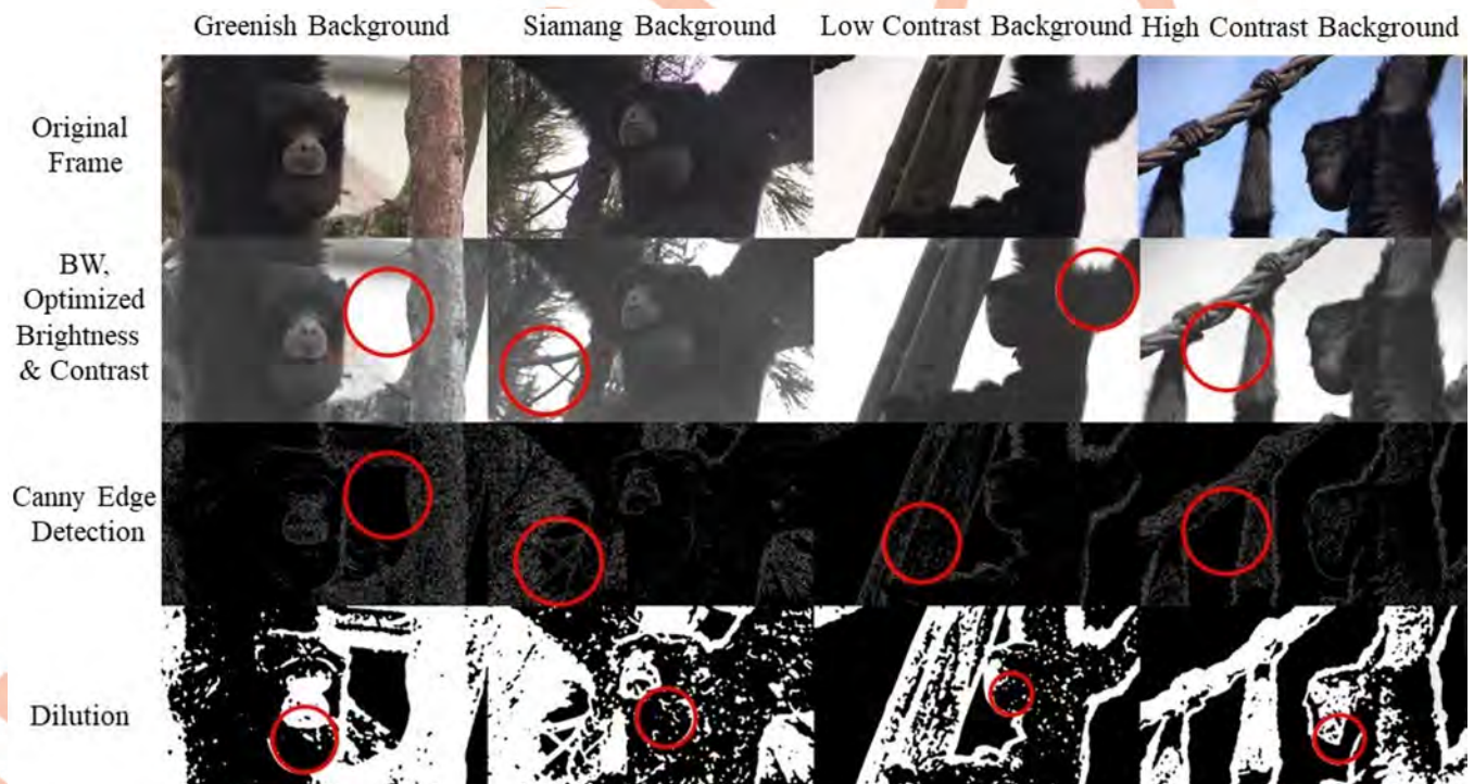
Fig 3. Image processing to increase Hough Transform circle detection success. Four pre-processing steps in four different frames with various backgrounds are shown to illustrate the necessity of the preprocessing steps for the Hough Transform approach to work. Only after the last pre-processing step are air sacs correctly found with the Hough Transform. All images are photos by Wim Pouw and Mounia Kehy.
