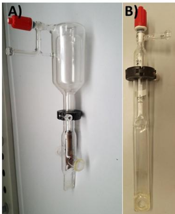
Figure 2. 4 A) Low temperature IR cell and B) room temperature IR cell adopted in this work for performing in situ IR experiments in the presence of probe molecules and/or reactants.
