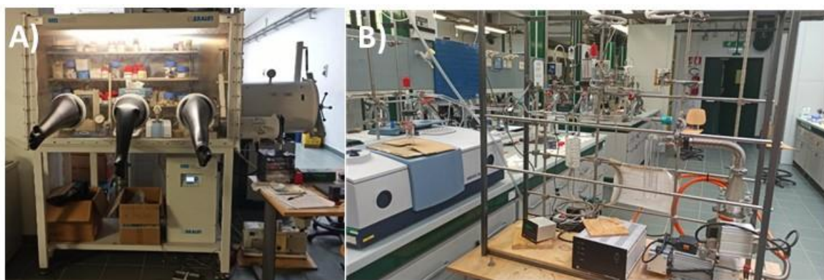
Figure 2. 3 A) The glovebox and B) vacuum line with cell connected while interfaced with IR spectrophotometer
