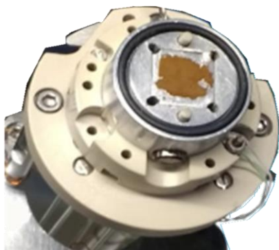
Figure 2. 6 The ambient pressure NEXAFS cell with the sample pressed inside indium plate
